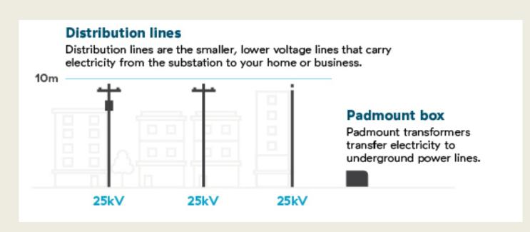
BC Hydro has approximately 55,254 kilometres worth of distribution lines (7200 volts) carrying the electricity to customers. These lines are either above ground or underground.
