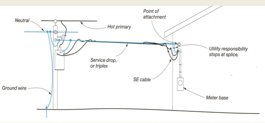
Notice the "Ground wire" attaching to the neutral wire at the power pole and then into the ground. This is to prevent electrocution.
