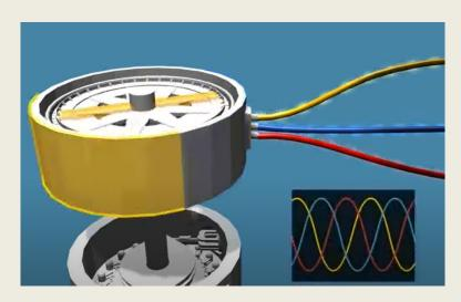
Falling water strikes a series of blades attached to a shaft which converts the kinetic energy to mechanical energy causing a turbine to rotate. The shaft is attached to a generator, which produces 3 phase electricity.
