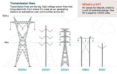
Grid transmission lines, usually supported by tall metal towers, carry high voltage electricity over long distances. The BC Hydro high-voltage transmission system consists of more than 18,286 kilometres of transmission lines, operating at voltages from 60 kV to 500 kV.
