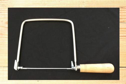
A coping saw is a small hand saw ideal for cutting straight lines and shapes including curves.
