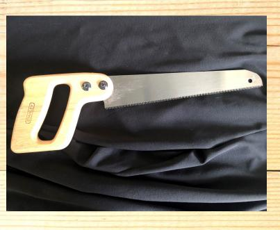
A hand saw is used for cutting straight lines in wood. Fingers MUST be at least 2" away from blade.
