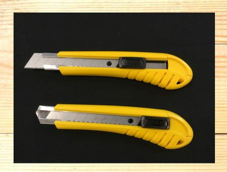
An exacto knife is a small retractable blade which can be used for cutting a variety of materials.
