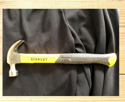
Hammer are used to attach wood pieces when used with nails. Place nail is location you want, hold the nail lightly with two fingers and lightly tap nail in. Then remove fingers and nail the nail into the wood with smooth stokes.
