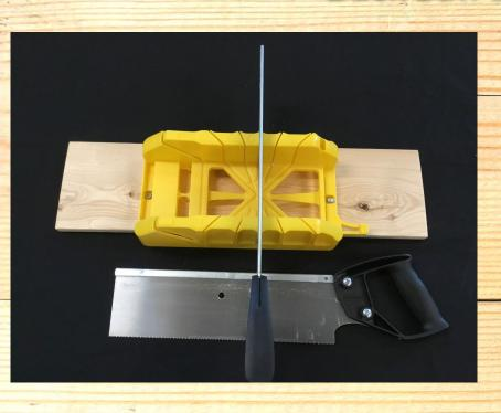
A backsaw is a large hand saw ideal for cutting straight lines and larger pieces of wood. It can cut on various angles when used with a miter box. Fingers must be at least 2 inches away from blade when cutting.
