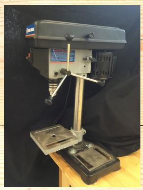
A drill press is a heavy duty power tool which is permanently attached to the work surface. It is used for drilling holes of various sizes.
