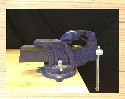
A vice is a clamp that is permanently attached to a workbench (Maker Cart).
