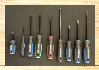
We have three different types screwdrivers in the tool car which match to different types of screws. They are flat head, Phillips head (cross shaped) and the Robertson h (square shaped) screwdrivers. Each type has different sizes and they are colour coded.
