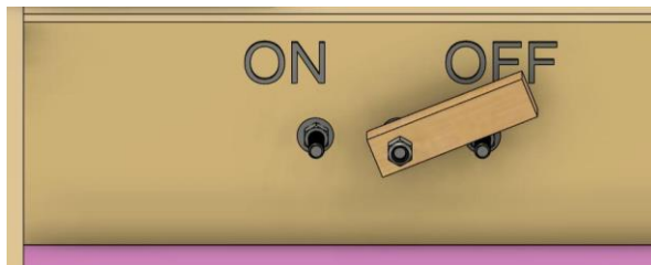
Figure: ECU Breaker Switch
